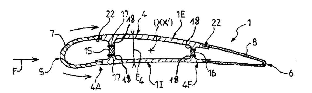
and added onto the downstream portion of the median module. Blades for rotating machines and corresponding fabrication methods.
