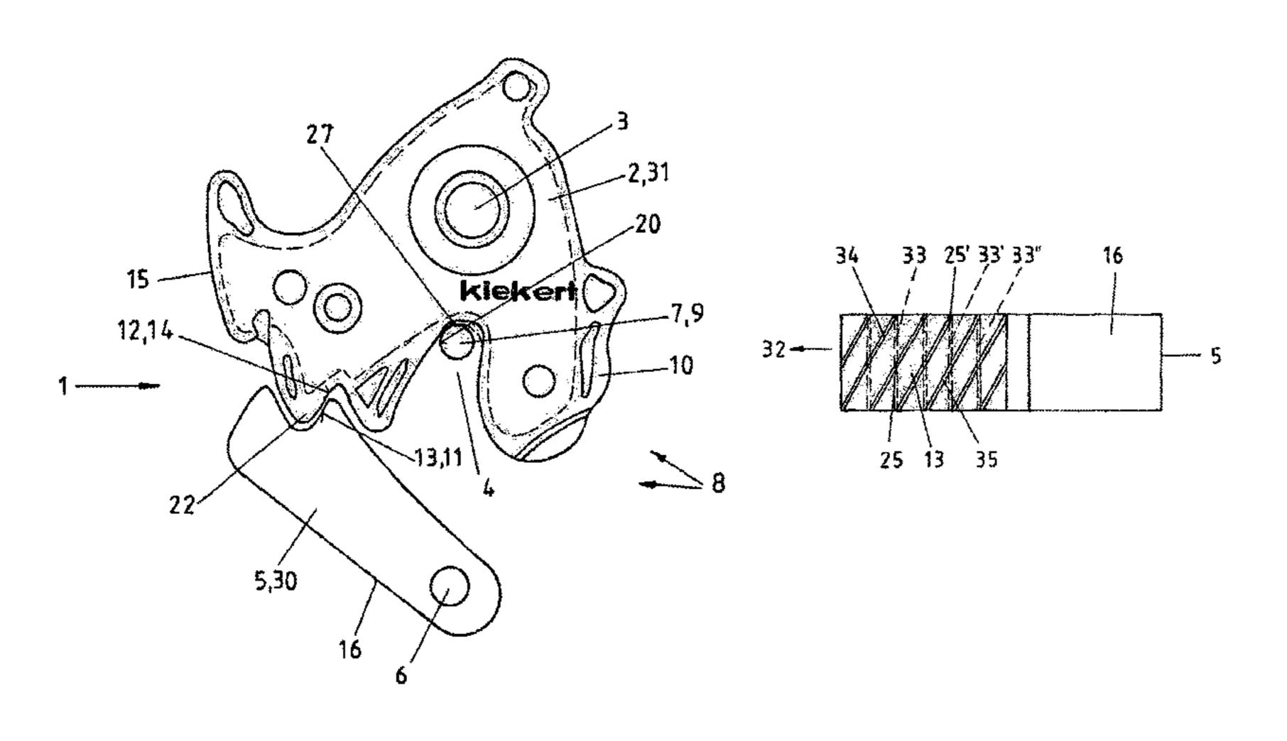
thereof, after stamping the pawl. Defined shapes of oblique channels and/or machining grooves are produced, for example, by milling out the machining grooves. The oblique machining grooves are produced at a defined angle and guarantee that the straight channels on the rotary latch only have a few overlapping points with the oblique grooves, if both locking parts come into contact with each other.
