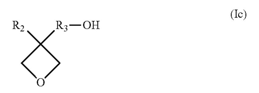
Examples of the diluent monomer having a hydroxyl group and an oxetanyl group include 3-methyl-3-oxet-anemethanol, 3-ethyl-3-hydroxymethyloxetane, 2-ethyl-hexyloxetane, and 3-ethyl-3{[(3-ethyloxetane-3-yl) methoxy]methyl}oxetane or the like.
