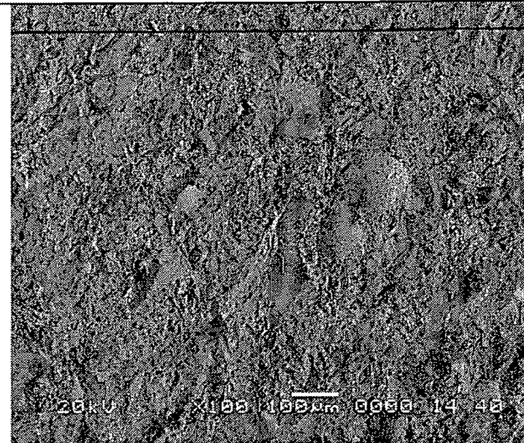
Figure 3 I SEM image with 100x magnification of the cross section of the sample of refractory composite material under examination: macroporosity.
