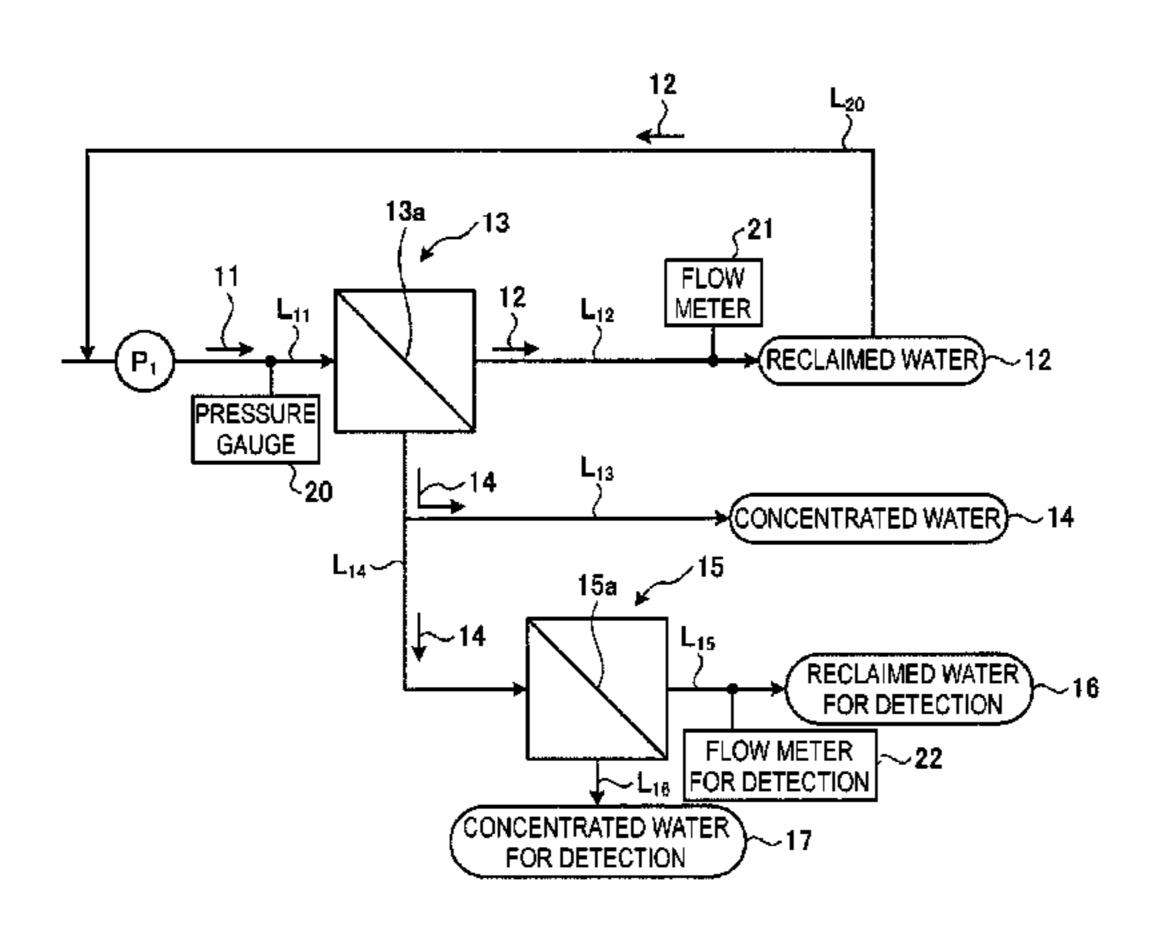
to obtain reclaimed water 12; and a scale detection unit 15 disposed in a branched line  $L_{14}$  branched from a concentrated water line  $L_{13}$  discharging concentrated water 14 having a high concentration of salt, the scale detection unit further concentrating the salt in the concentrated water 14 to obtain reclaimed water for detection 16, and including a detection membrane 15a detecting the absence or presence of scale component deposition in the concentrated water 14.
