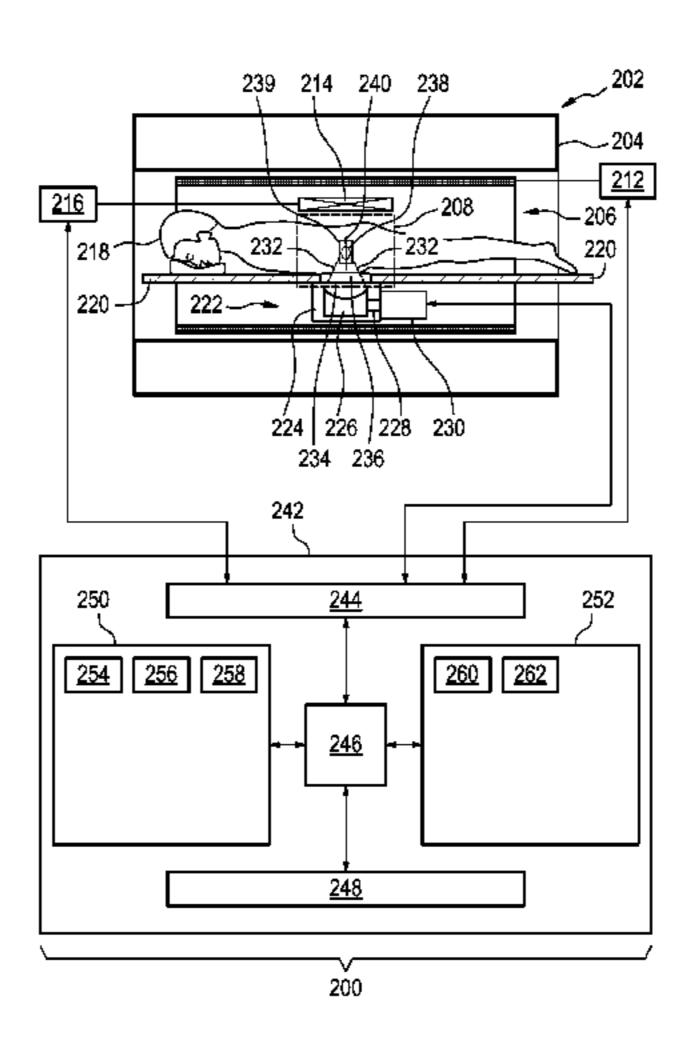
(102) the high intensity focused ultrasound system to sonicate the target zone during the acoustic radiation force imaging pulse sequence and reconstruct (104) a radiation force image (258) using the magnetic resonance data.
