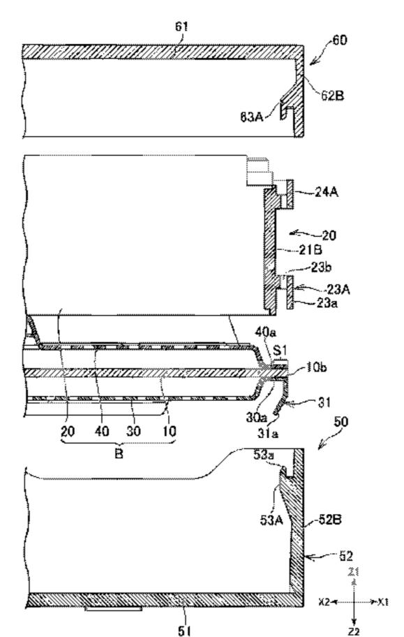
when the lower cover (50) and the inner part (B) are combined together in the vertical direction, the guide section (31) comes into contact with a right wall section (52B) of the lower cover (50) and pushes the right wall section (52B) rightward so as to cause the first engaging section (53A) to move rightward beyond the first edge section (S1).
