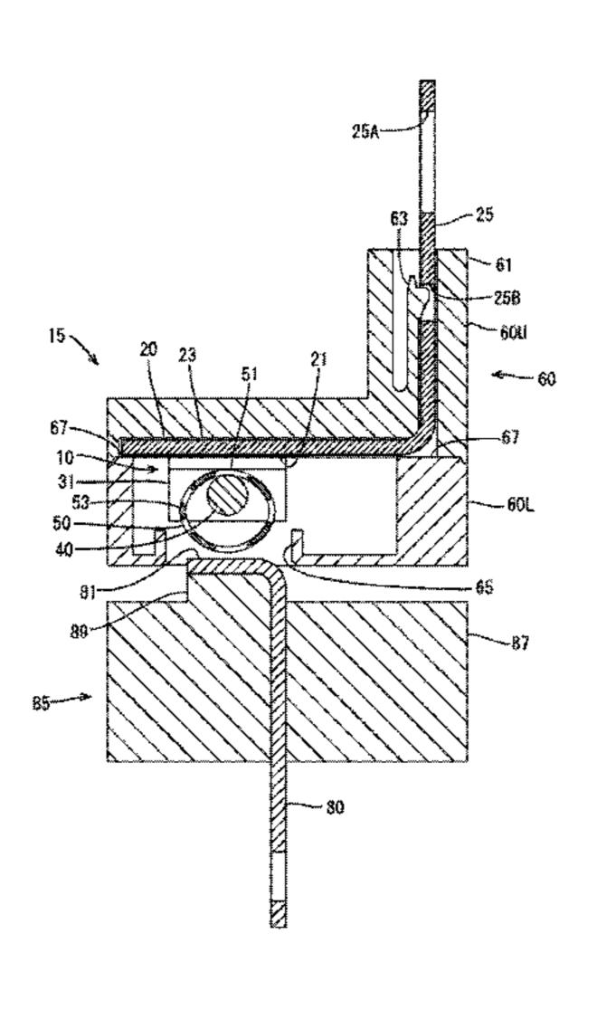
the mating terminal (80) and the electrical contact member (20) approach each other. A holder shaft (40) is inserted in the canted coil spring (50) to hold the canted coil spring (50) in a posture where the coil axis L is parallel with the facing surface (21) of the electrical contact member (20).
