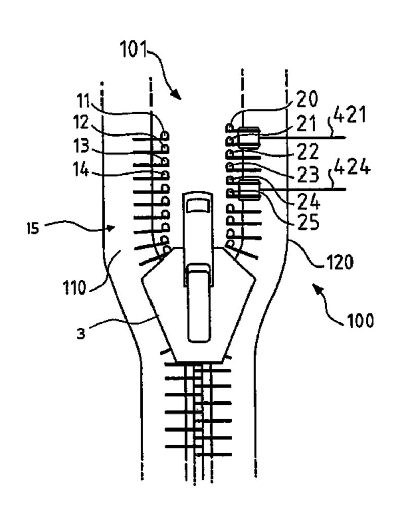
of said detected continuity state. The first terminal (21) and the second terminal (24) are spaced apart from each other by at least one tooth (22, 23), said at least one tooth having no electrical connection with said terminals when the teeth of the two rows are in the separated state.
