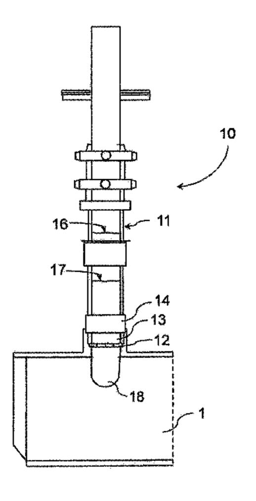
received from the laser devices is used for calculation of the distances of the levels of the raw paste and molten paste from the contact shoe ring.
