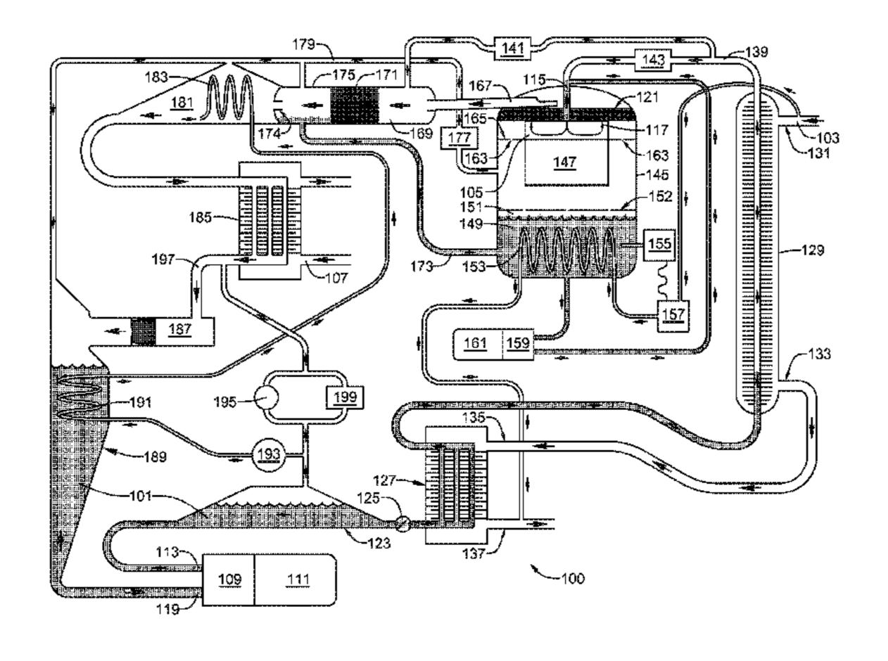
positive-displacement hydraulic pump, which provides continuous flow of the organic refrigerant in the liquid phase from the low-pressure zone to the high-pressure zone, the hydraulic pump and the positive-displacement decompressor maintaining a pressure differential between the two zones of between about 20 to 42 bar.
