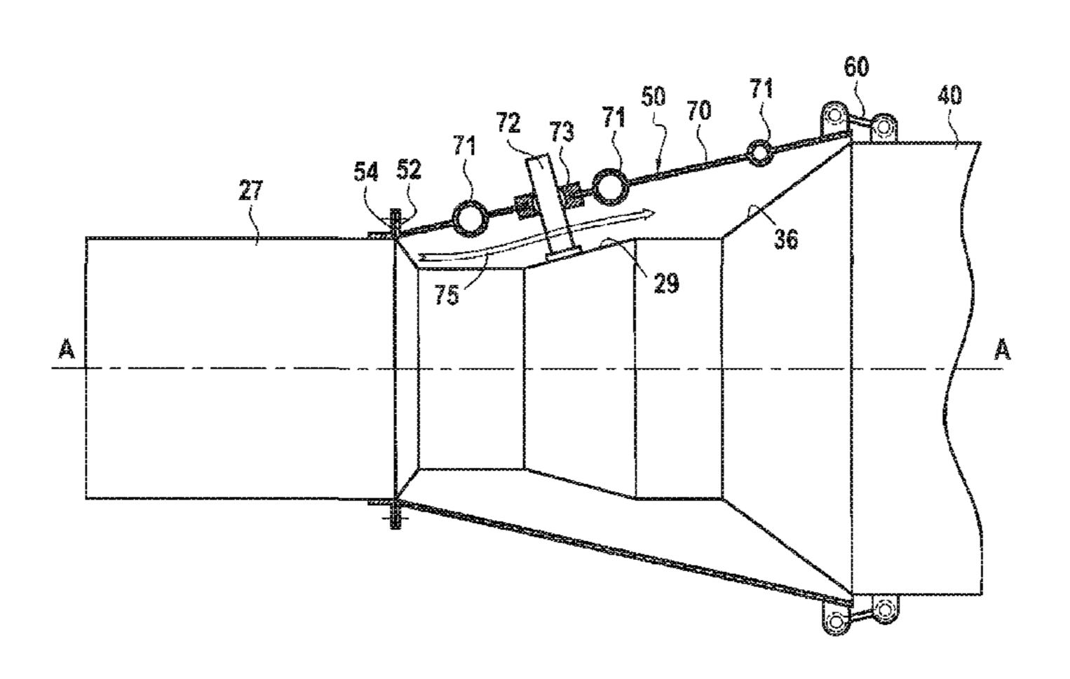
the first casing, second attachment zone mounted on the second casing, and a wall provided between the first and second attachment zones and surrounding the third casing, wherein the reinforcing shell further includes at least one pipe segment integrated in the wall.
