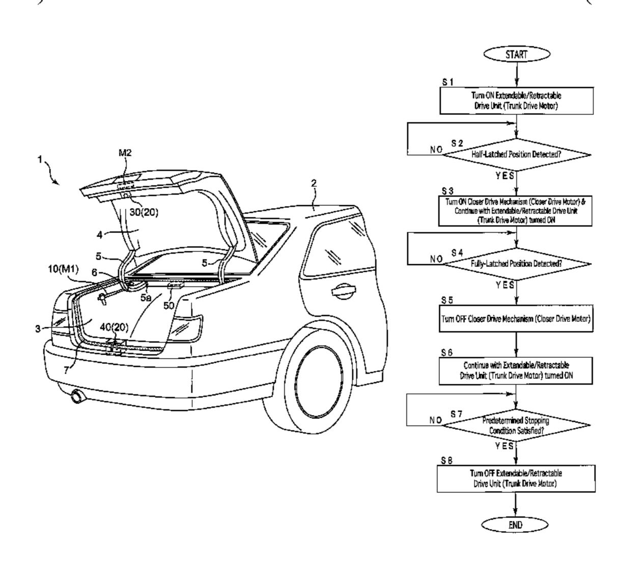
driver ends operation and the first driver continues to drive the opening-and-closing body in the closing direction until the stop detector detects that the predetermined stopping condition is satisfied.
