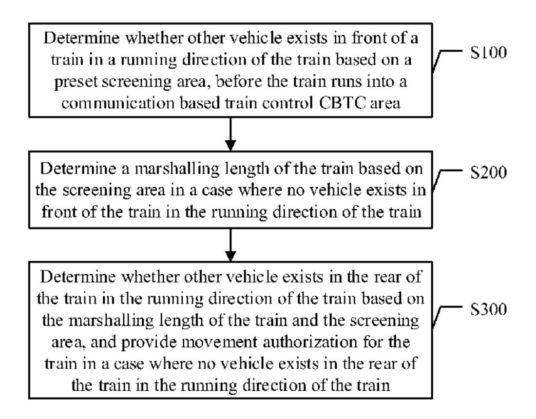
length of the train and the filter area, whether any other vehicle exists behind the train in the travel direction thereof, and if no other vehicle exists behind the train in the travel direction thereof, providing the train with a movement authorization.
