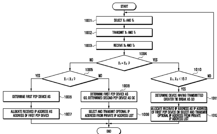
address to be allocated to the group client to the external terminal from the wireless terminal.
