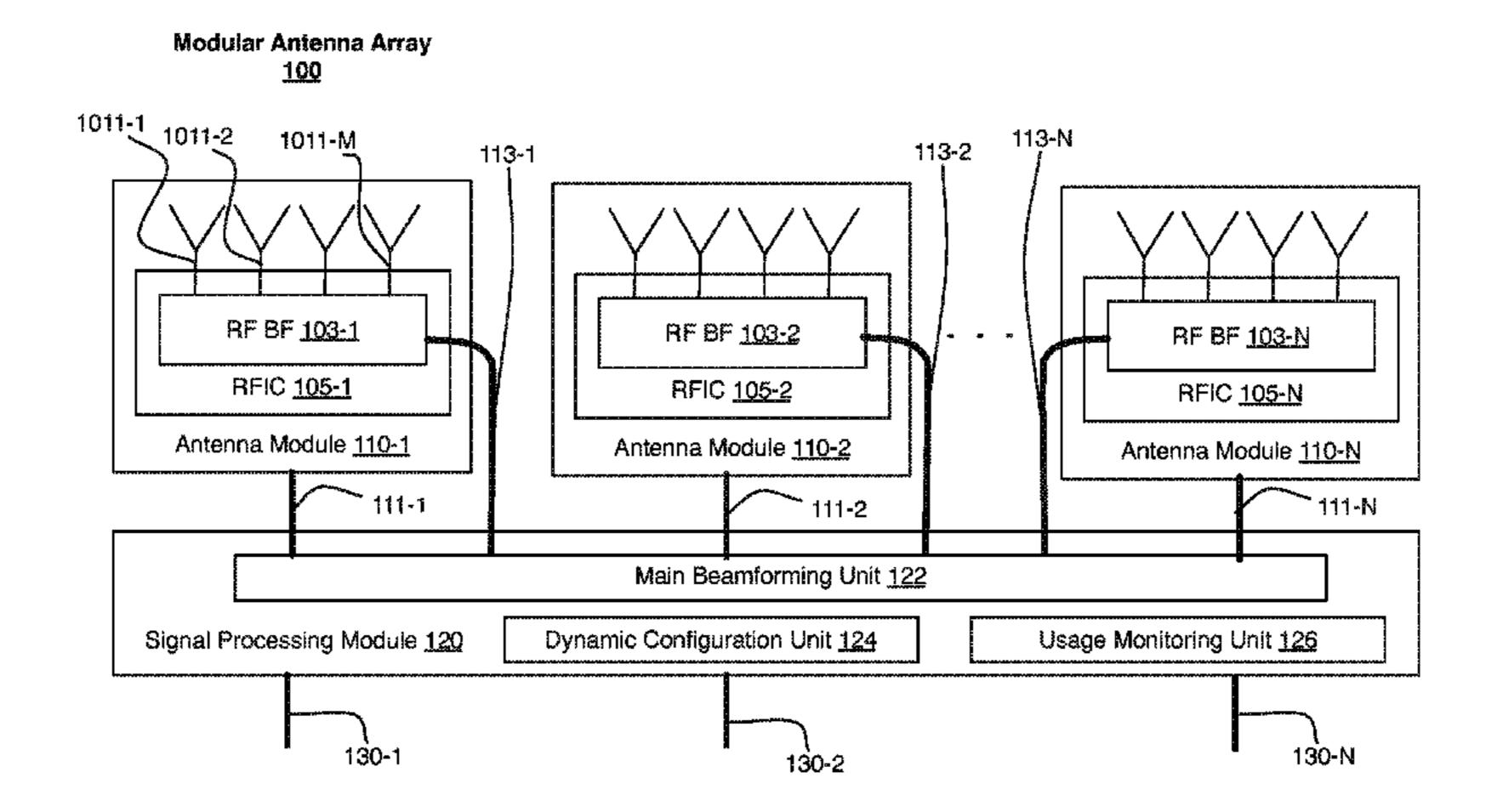
modules, and a main beamforming unit coupled to the dynamic configuration unit and each of the antenna modules, the main beamforming unit to generate signal adjustments relative to the one of the plurality of antenna modules to control the antenna beam associated with the one of the plurality of antenna modules based at least in part on the usage.
