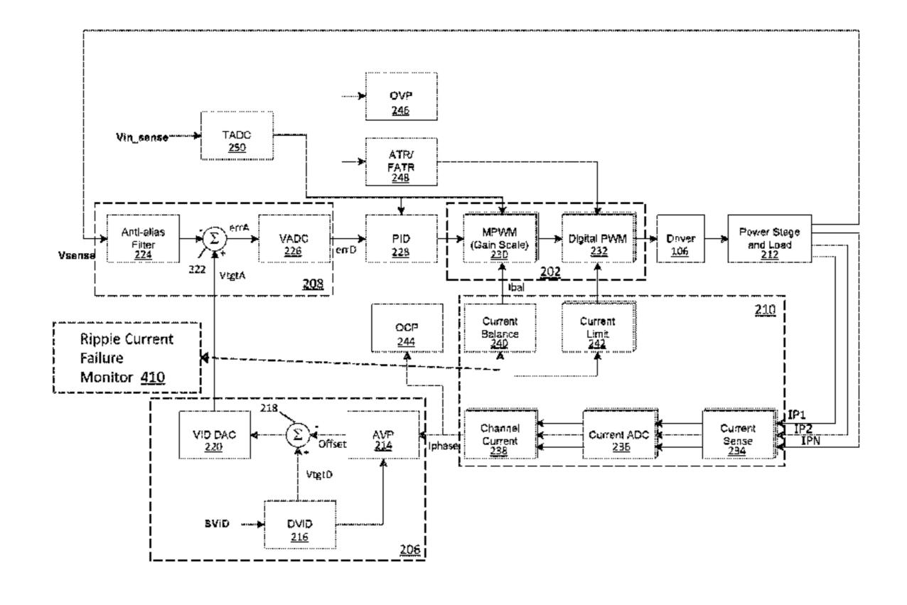
ripples in the phase currents, and detect if any of the phase currents fail to have a ripple current pattern that matches an expected ripple current pattern.
