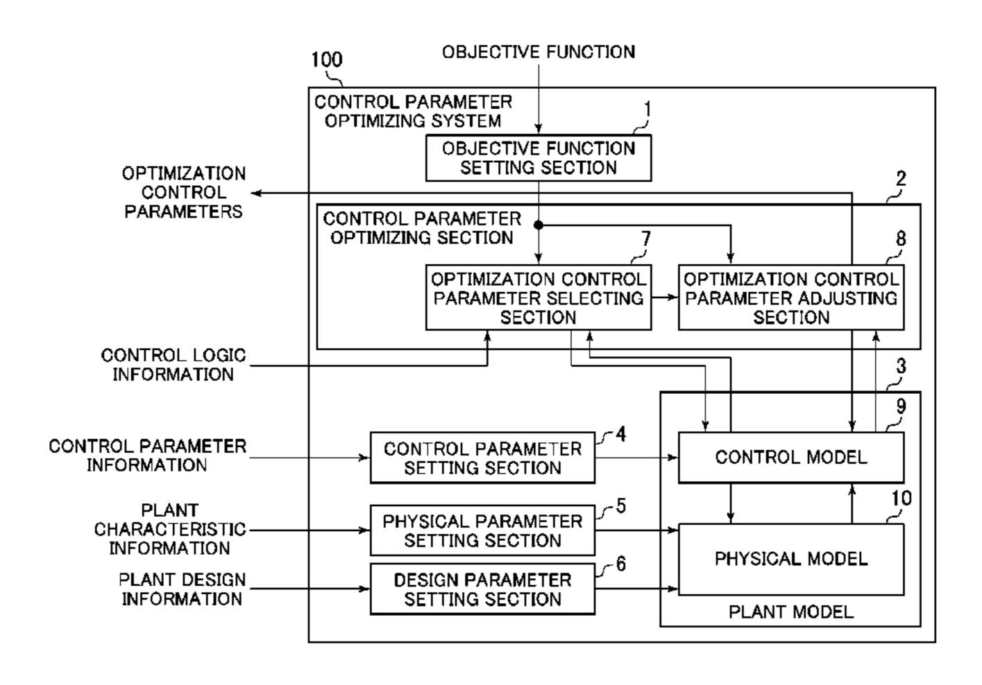
optimizing an objective function based on control logic information extracted from a power plant. The optimization control parameter adjusting section adjusts the value of the optimization control parameter using the plant model in such a manner as to optimize the objective function.
