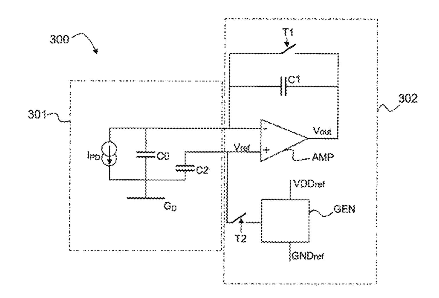
Isolating the second input of the amplifier (AMP) from the voltage source (GEN); and Integrating the current generated by the set (301) of photodiodes.
