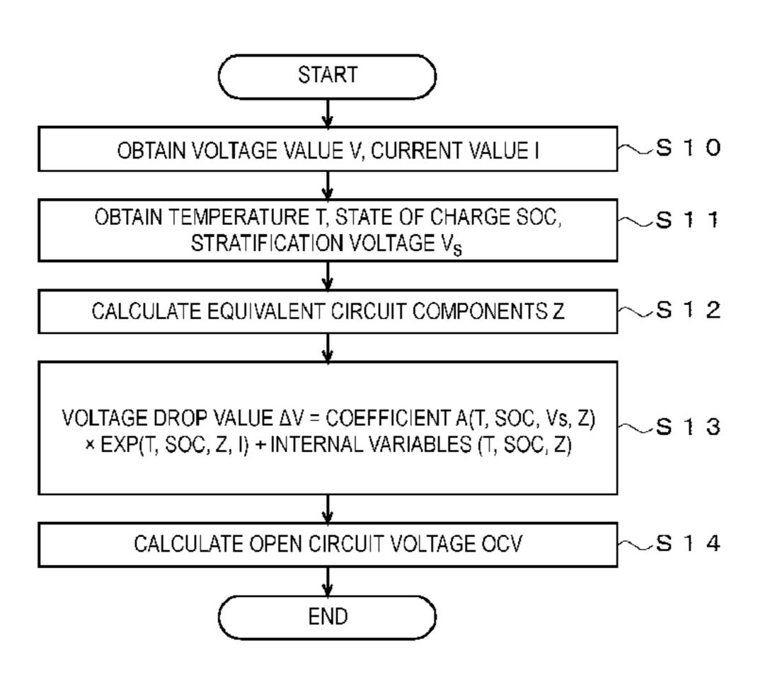
corresponding to the equivalent circuit component calculated by the calculating unit and having an element value varying nonlinearly in accordance with the value of the dark current; and a state detecting unit (an open circuit voltage calculation module (118)) that detects a state of the secondary battery on the basis of the value of the voltage drop estimated by the estimating unit.
