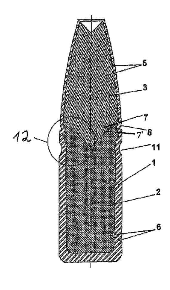
has a peripheral break away edge on the outer circumference in the region of the predetermined breaking point.
