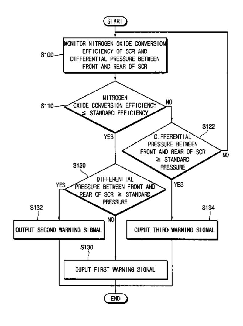
first warning signal when the detected differential pressure is lower than a predetermined pressure.
