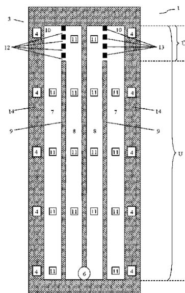
by means of primary combustion is completely combusted in the lower oven by means of secondary combustion. The transition region in which the gas is deflected in the lower oven may be divided into a plurality of flow channels.
