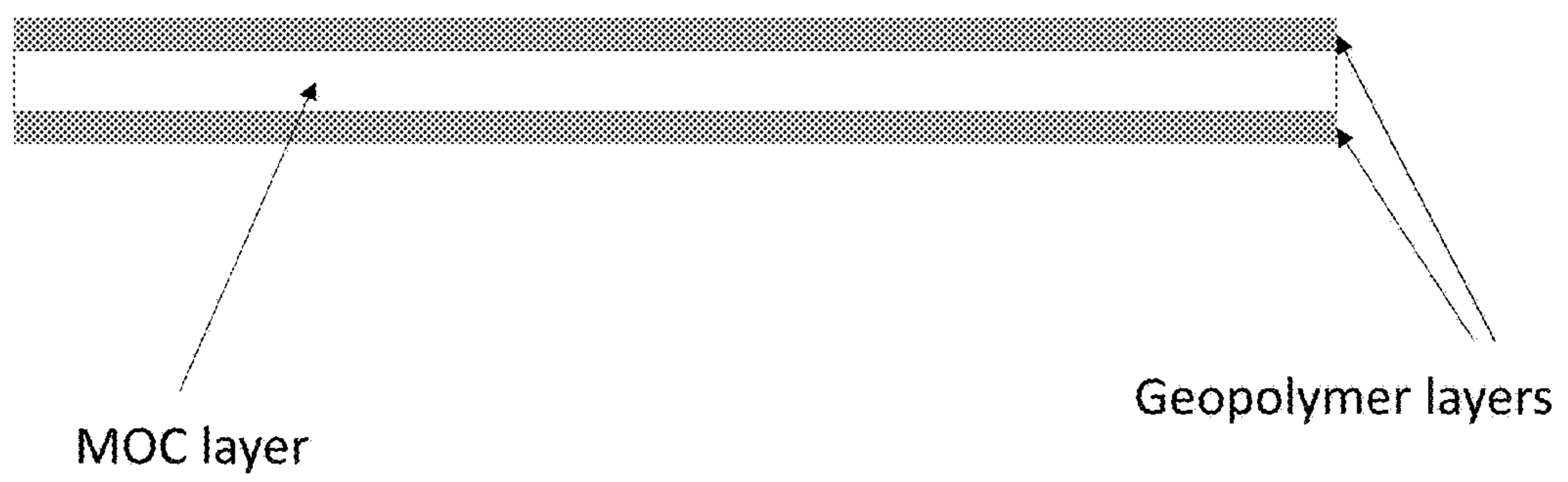
Figure 3. Cross-section structure of a sandwich board with MOC core
