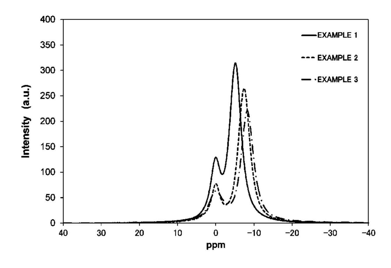
this embodiment includes a carbon structure which has a ratio of an ultramicropore volume to a micropore volume of 60% or more, and in which stored hydrogen exhibits, in <sup>1</sup>H-NMR measurement, a second peak at a position corresponding to a chemical shift of from -2 ppm to -20 ppm with respect to a first peak attributed to gaseous hydrogen.
