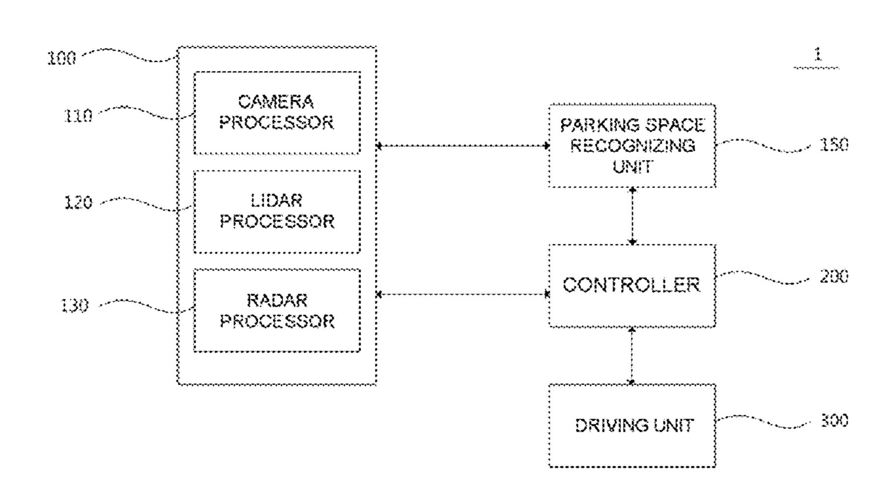
A controller calculates a moving path between a current position of the subject vehicle and an optimal parking area and operates the subject vehicle based on the moving path.
