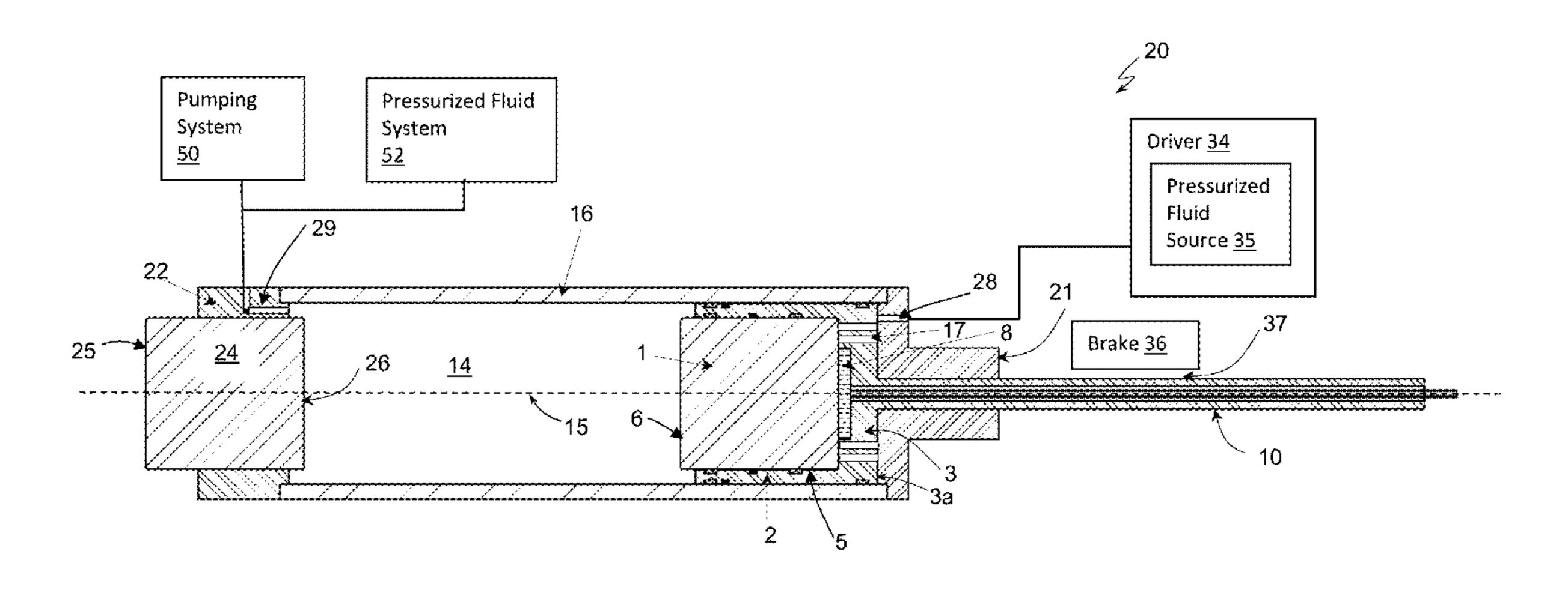
motive force to the sabot. Once accelerated within the inner bore of the housing the sabot can be decelerated by applying a restraining force to the sabot while the piston can be released at least partially from the sabot to continue to move toward the transducer until it impacts the transducer. Examples of methods of operating the pressure wave generator are disclosed.
