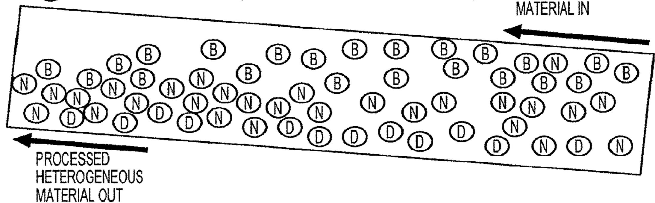
MICROWAVE - TRANSPARENT CONDUIT DETAIL WITH PREFERABLY HEATED CARRIER FLUID WITH UNIFORMLY INCREASING TEMPERATURE (AND DECREASING DENSITY) AND INDIVIDUAL PARTICULATE COMPONENTS WITH DIFFERENT DENSITY RANGES
