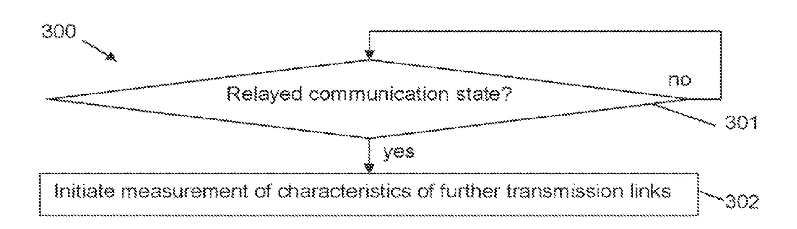
communication state is determined (301) and a measurement of characteristics of further direct radio transmission links between the user equipment (106) and the wireless radio network (100) is initiated (302) depending on the relayed communication state.
