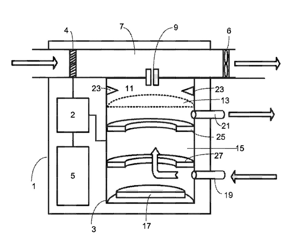
collecting a flow of air to be tested by the spectrometer (3); a heater (4) configured to heat the air to be tested to vaporize an aerosol carried by the air and a controller (2) configured to control the spectrometer (3) to obtain samples from the heated air, wherein the controller is configured to increase a heat output from the heater (4) for a selected time period before obtaining samples from the heated air.
