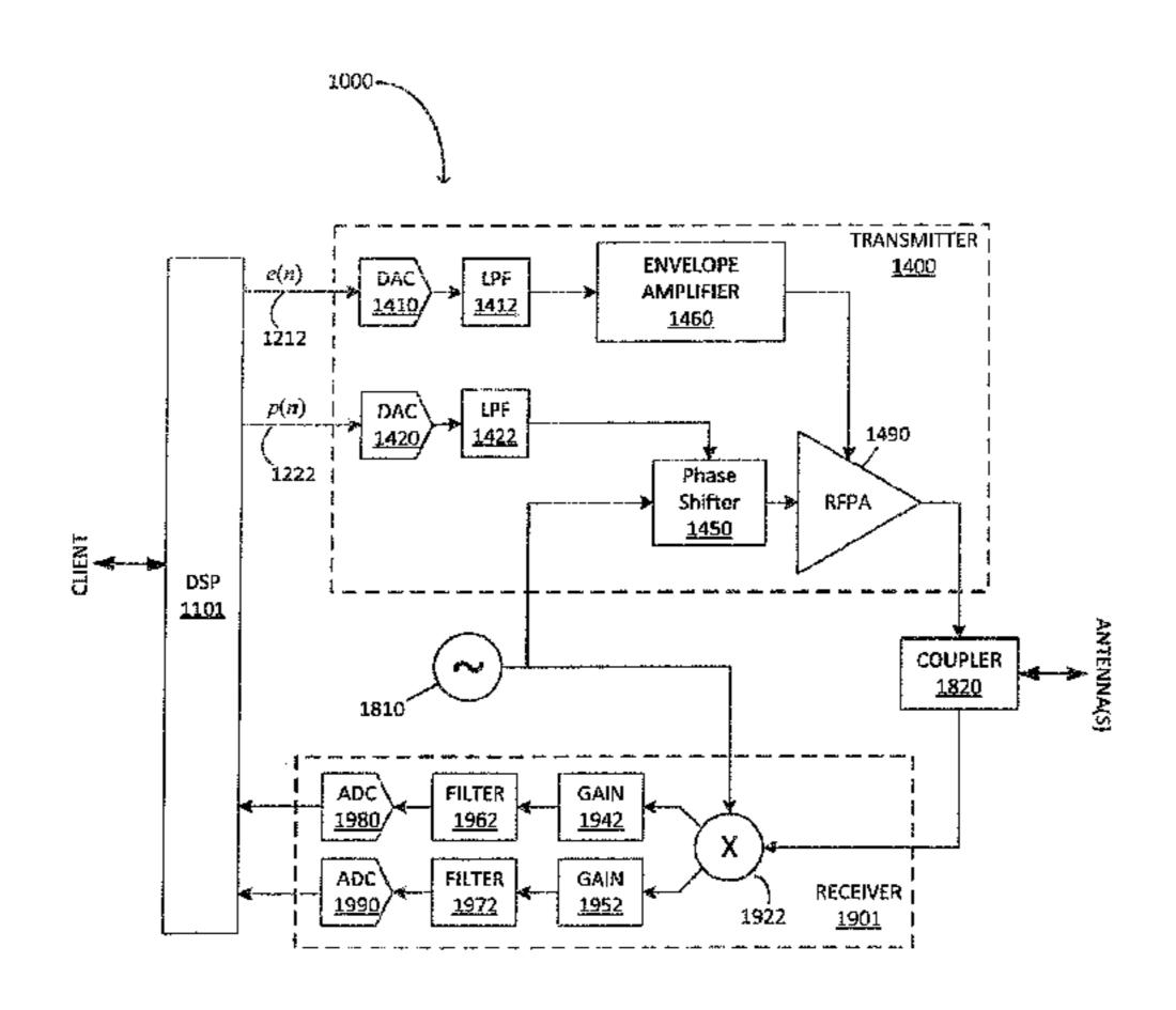
OPR-ASK signals to reduce AM modulation depth and provide a continuous phase signal for the phase modulator.
