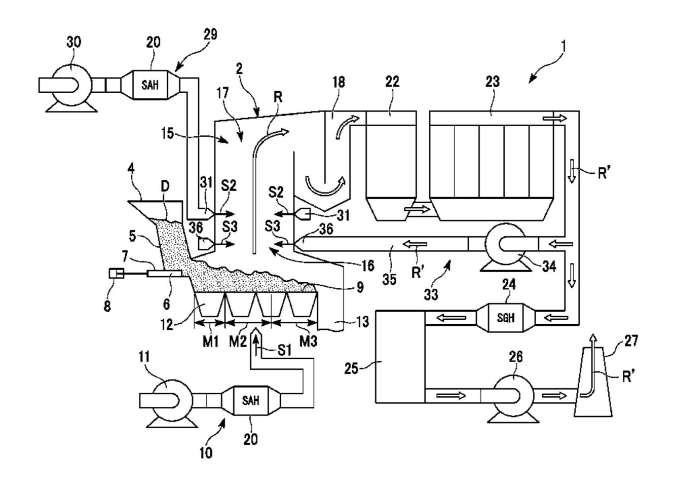
channel via a secondary combustion air nozzle provided on the combustion gas channel, in which the recirculated exhaust gas nozzle and the secondary combustion air nozzle are arranged in different positions in a plan view.
