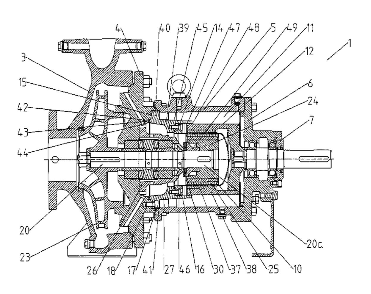
axis, an inner rotor arranged at an end of the impeller shaft opposite the impeller end, an outer rotor which interacts with the inner rotor, and an adapter element which connects the split case to the pump housing or to a component paired with the pump housing, in particular a housing cover. The adapter element includes a mounting flange which rests against a support surface of the pump housing, in particular of the housing cover (4), on a face adjacent to the interior.
