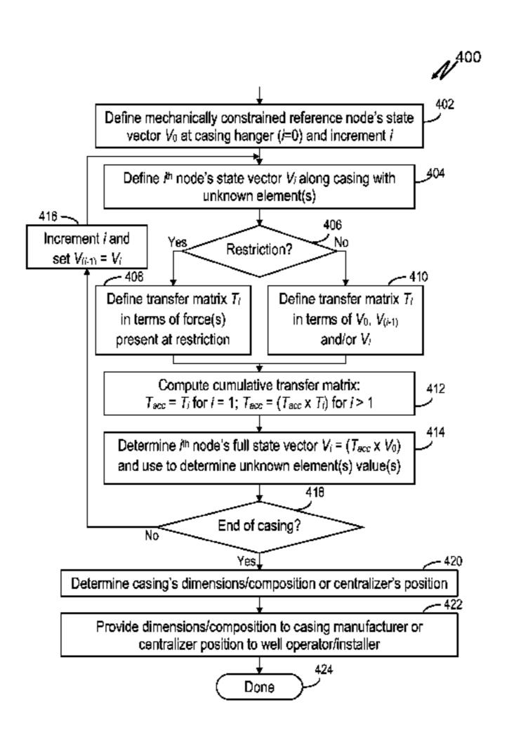
state vector describing a corresponding node position and one or more forces present at said node. The method further includes applying the transfer matrices to obtain each of the state vectors' values, deriving from at least one of the state vectors a parameter value for said component, and specifying a component having said parameter value. The parameter value can include a centralizer or stabilizer composition, manufacturing dimensions, or position.
