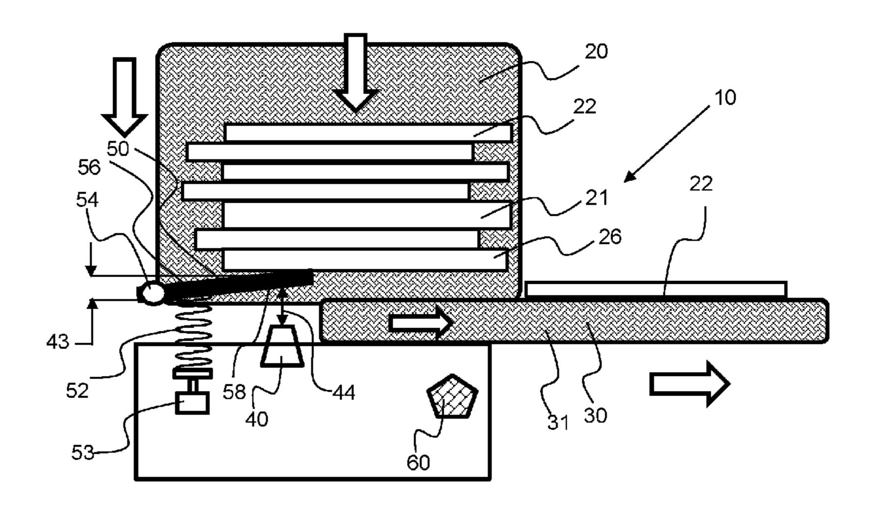
have a low friction surface to allow the mail to slide into the conveyor and an optical surface to allow reliable optical sensor detection of the optical panel position.
