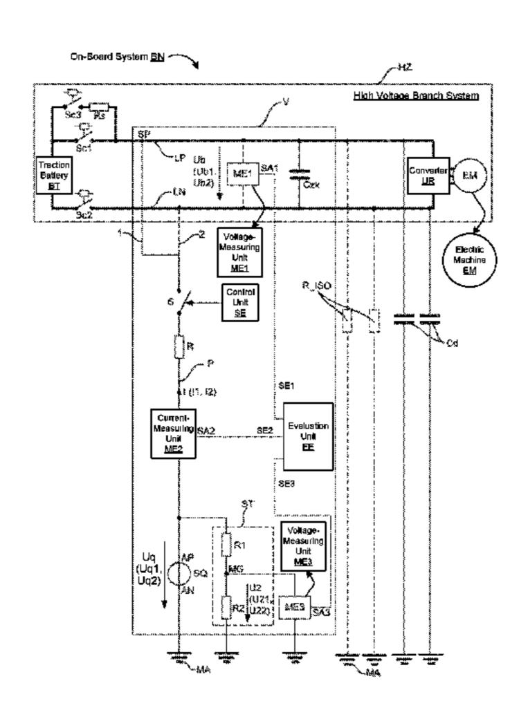
current measurement values of the current-measuring unit, and the first and the second voltage value.
