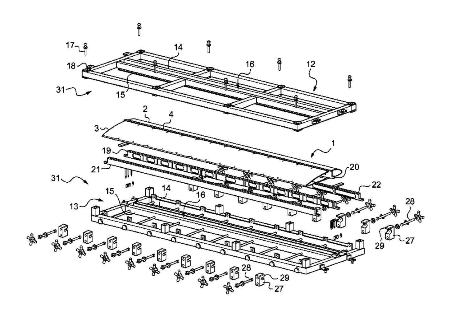
parts disposed. The set of preformed parts is held in a welding position with the clamp and framework while a welding operation is performed.
