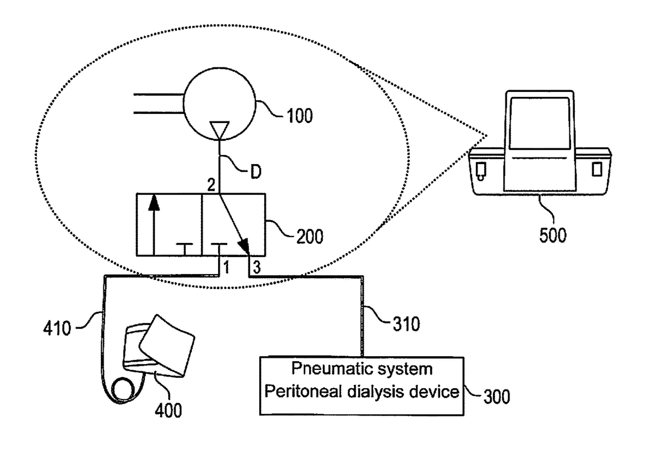
The present invention relates to a dialyzer, in particular to a peritoneal dialyzer, comprising at least one compressor and comprising at least one pneumatic consumer which is in 5 communication with the compressor such that it can be acted on by compressed air from the compressor.
