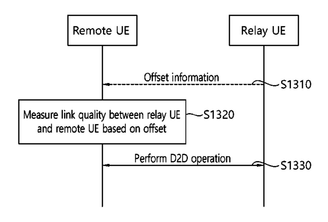
for the remote UE on the basis of the measurement, wherein the offset is determined on the basis of information which may have an effect on communicating with a base station by the remote UE through the relay UE.
