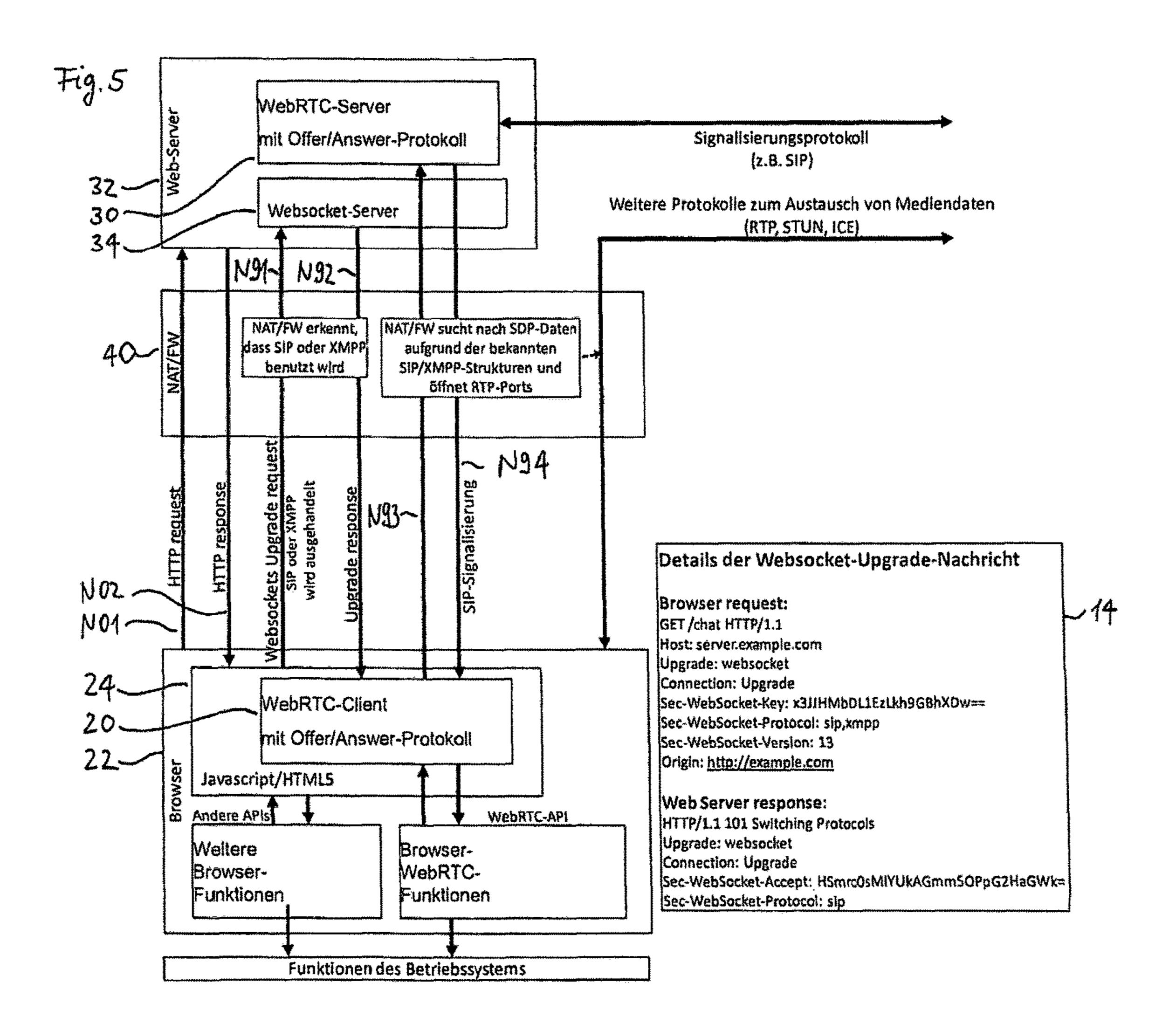
TELECOMMUNICATION SYSTEM AND METHOD FOR TRAVERSING AN APPLICATION LAYER GATEWAY FIREWALL DURING THE ESTABLISHMENT OF AN RTC COMMUNICATION CONNECTION BETWEEN AN RTC CLIENT AND AN RTC SERVER
