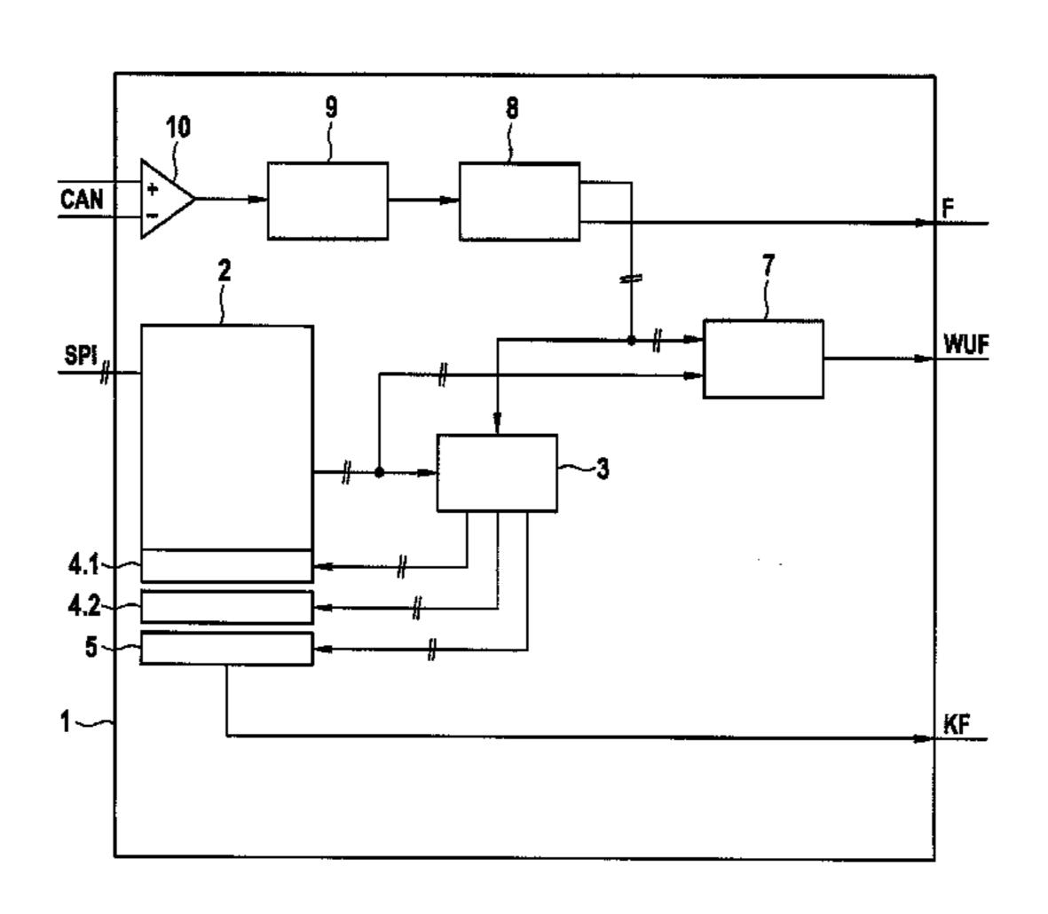
and compared with the checksum stored in the reference register. If the recomputed checksum does not match the stored checksum, a wake-up process is triggered.
