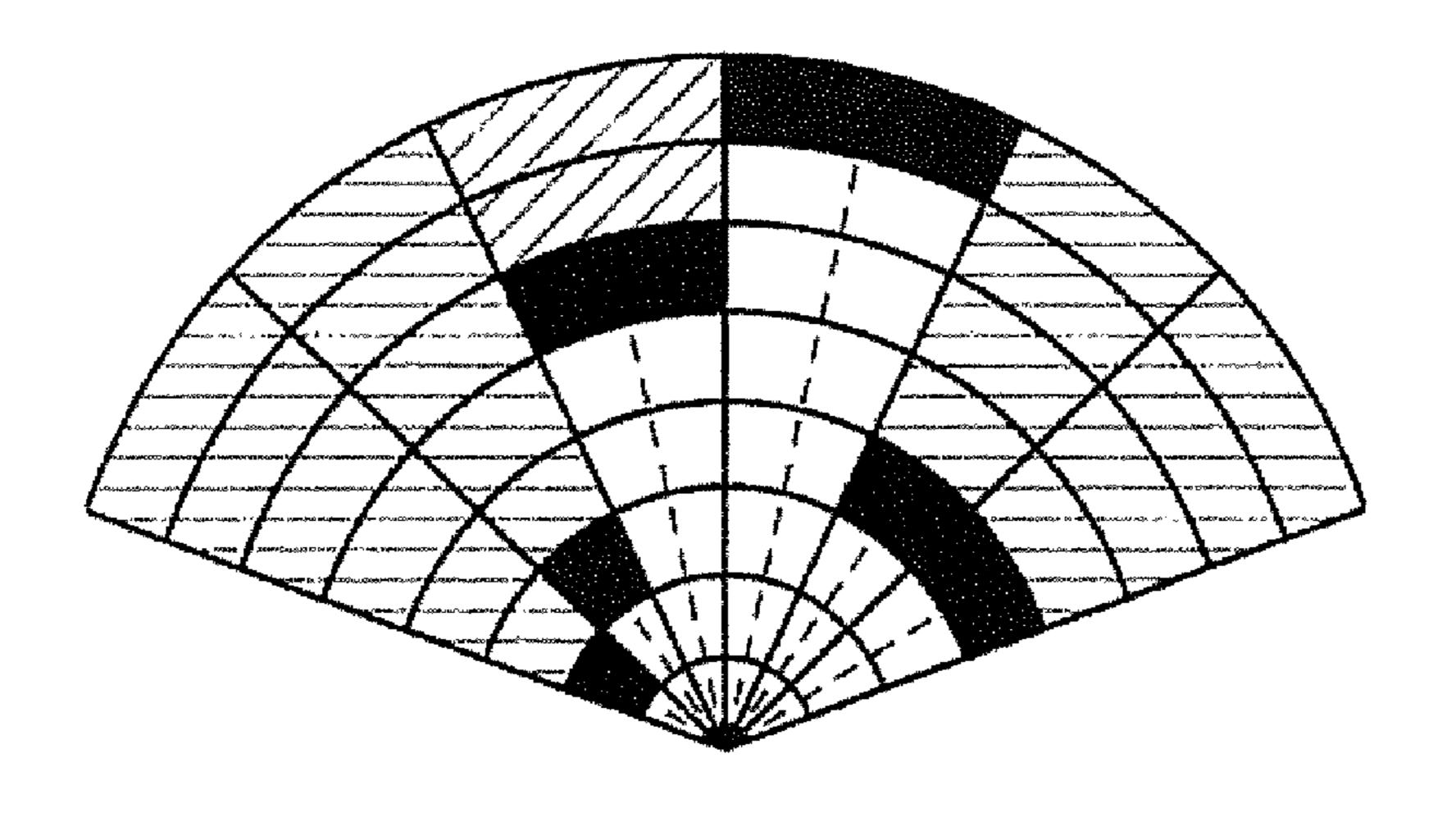
location module (16) designed to determine the position of the vehicle in the environment, which maximizes a measurement of correspondence between the measurement values  $(M\_SCAN_{t,i})$  and the built values  $(M\_GRI_{t,k})$ . The invention also describes an associated method.
