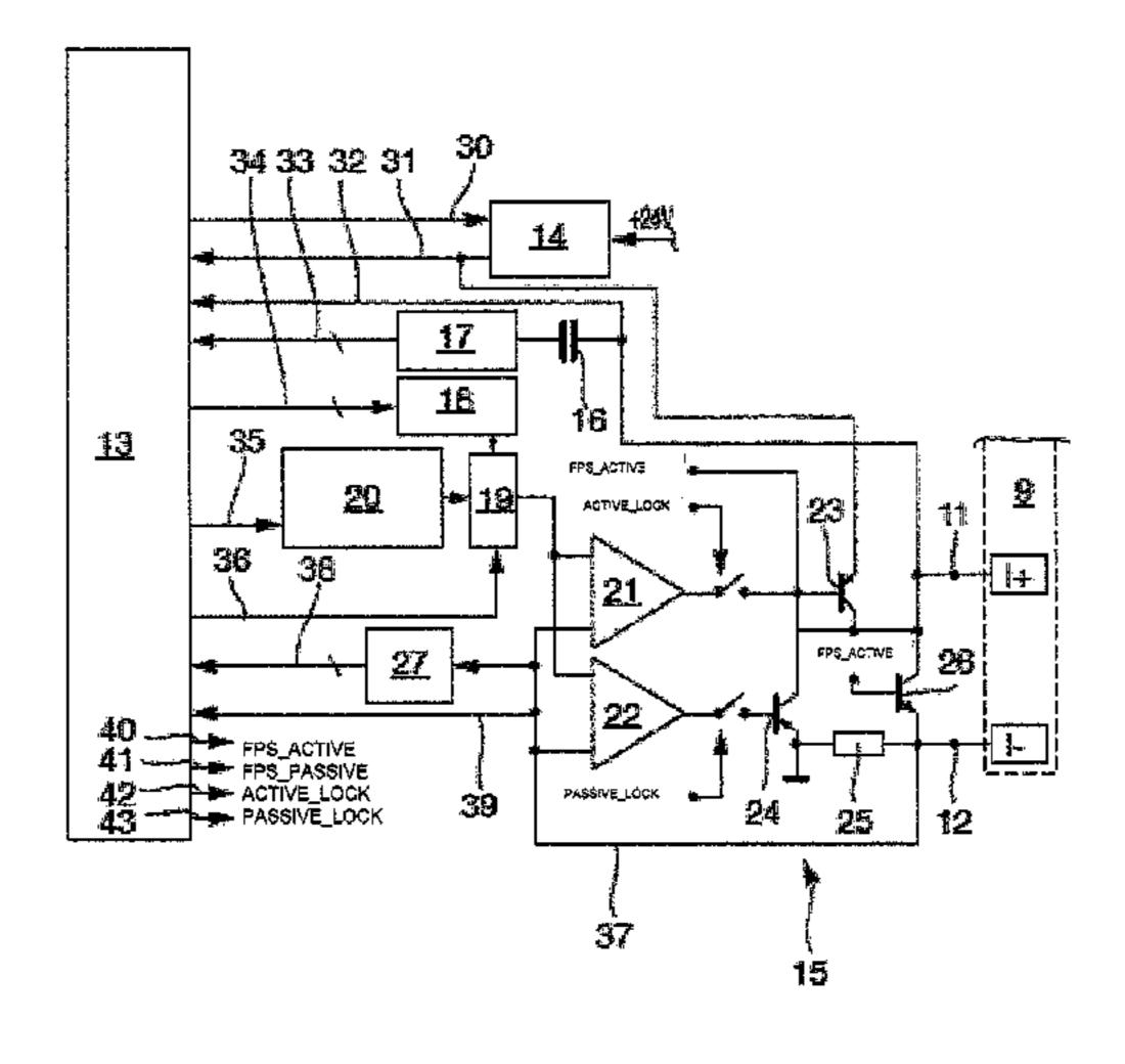
circuit an output current can be set with an electrical current level in a first interval for the LOW state and in a second interval for the HIGH state.
