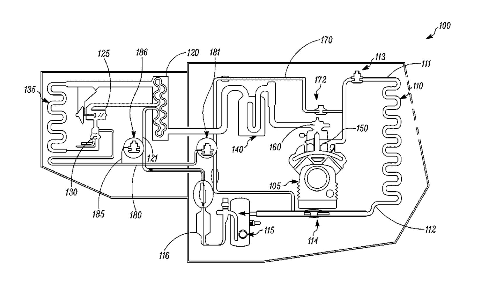
refrigerant trapped in the liquid refrigerant section and/or the condenser coil into the heating/defrost branch of the TRU, which may include an evaporator coil, an accumulator tank and/or associated refrigerant lines.
