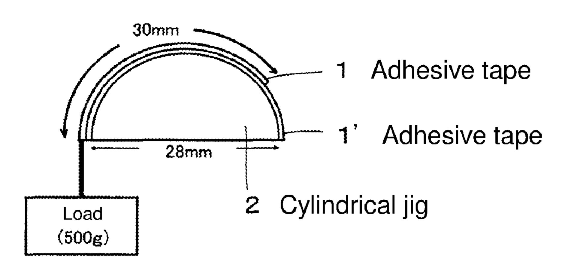
environment for 30 minutes, and a check is performed to determine whether or not the weight has fallen due to separation of the adhesive tape 1.
