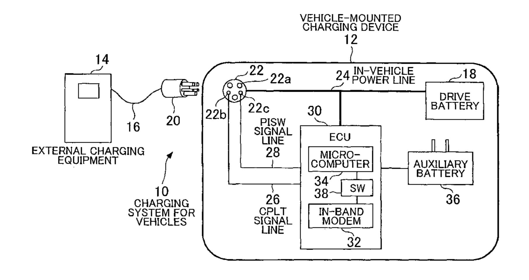
vehicle-mounted electronic control unit is configured to perform charging communication, relating to charging of the vehicle-mounted battery, with the external charging equipment using an in-band modem (32). The modem startup control unit starts up the in-band modem when the vehicle-mounted electronic control unit performs the charging communication, and that stops a startup of the in-band modem when the vehicle-mounted electronic control unit does not perform the charging communication.
