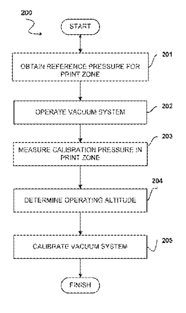
calibration pressure value and applying an operating setting to the vacuum system based on the determined altitude.
