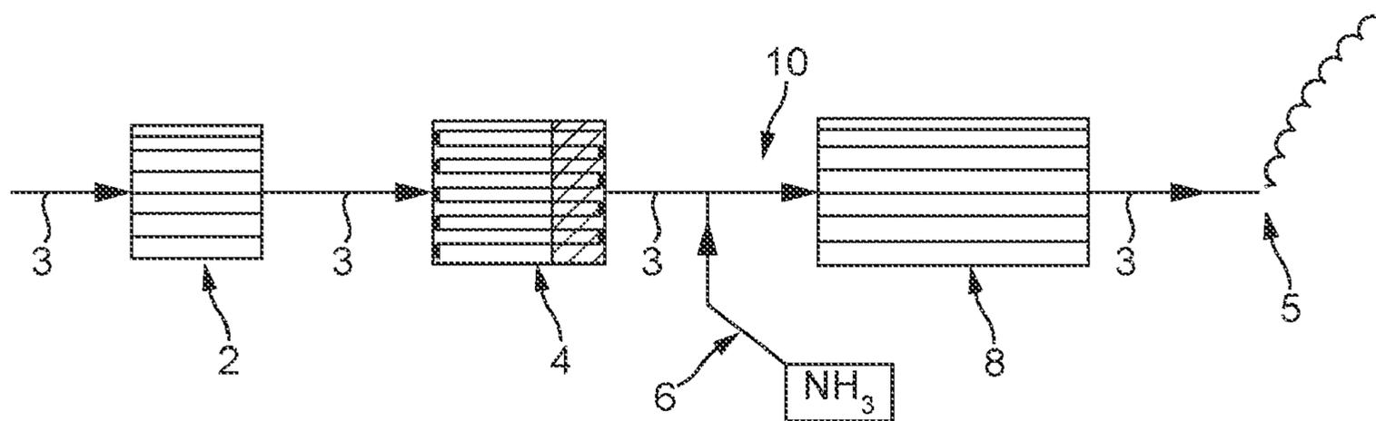
strate monolith comprising an oxidizing catalyst on a substrate monolith for use in treating exhaust gas emitted from a lean-burn internal combustion engine. In particular, the invention relates to a catalyzed substrate monolith comprising a first washcoat coating and a second washcoat coating, wherein the second washcoat coating is disposed in a layer above the first washcoat coating.
