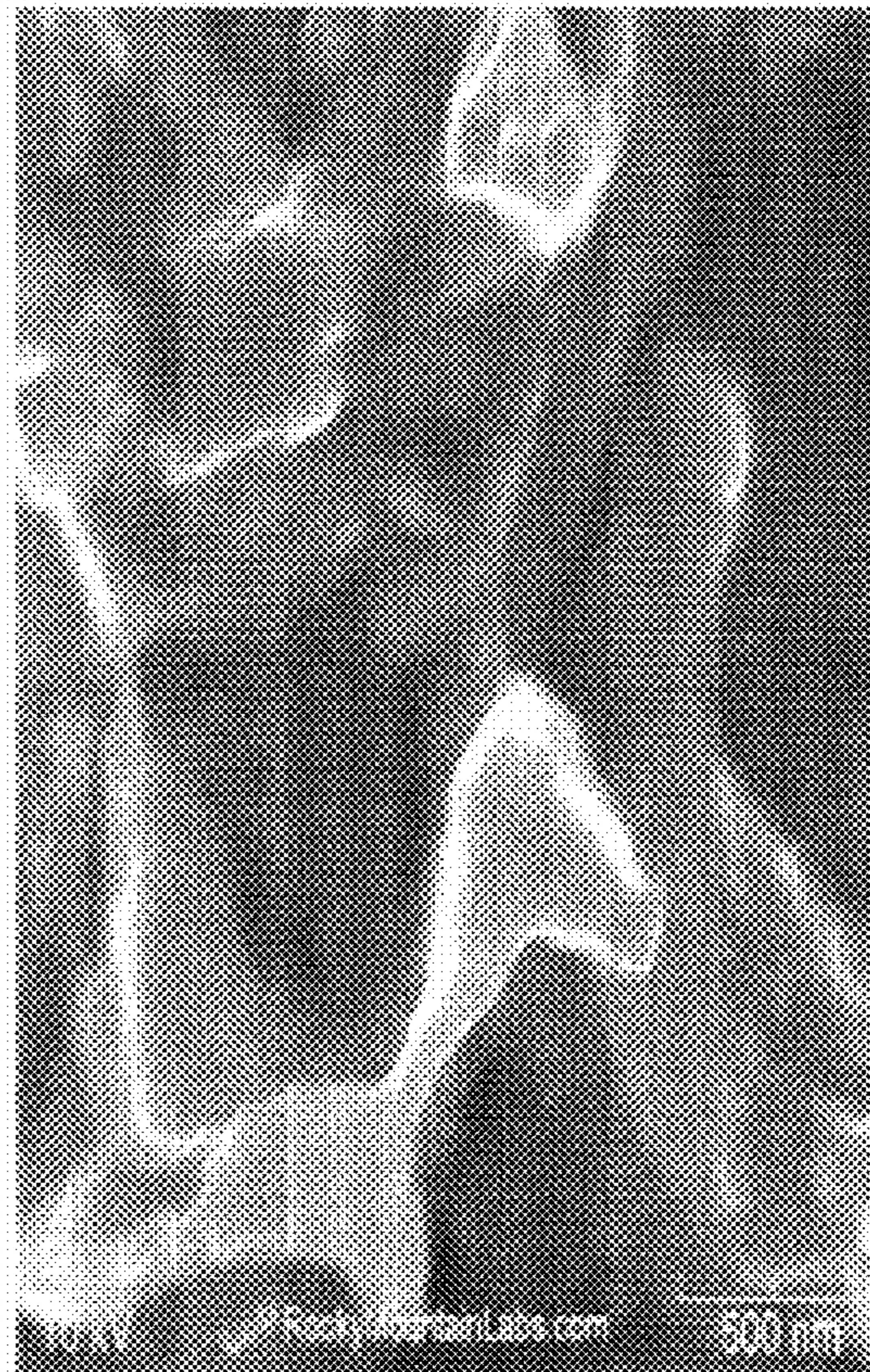
Fig. 4D Conventional micro-etched rough copper surface
