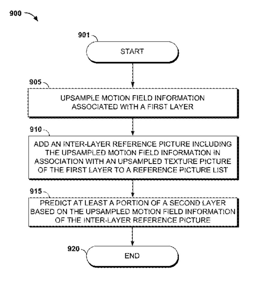
first layer to a reference picture list to be used for inter prediction. The processor may encode or decode the video information.
